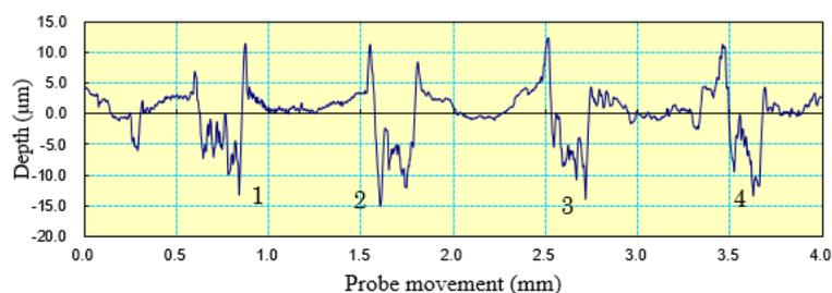
Fig 2: Depth profile of 10% density textured specimen
