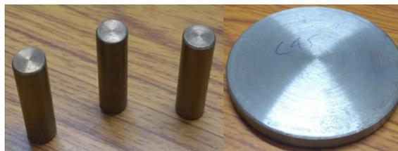
Fig 1: Pin and disk specimens
